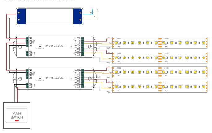
2. When total load of each receiver is over 10A
