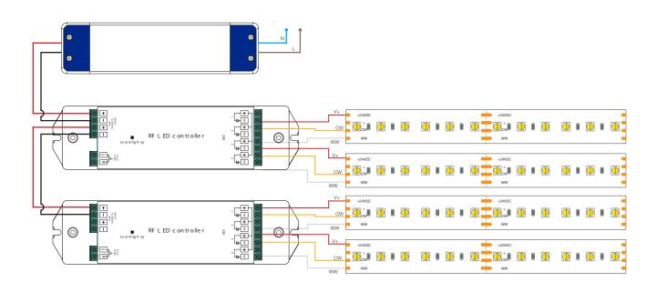
2. When total load of each receiver is over 10A
